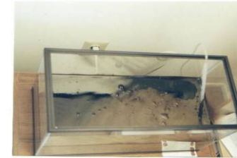
Photograph showing dispersion of bilge oil after 48 hours of SpillRemed (Marine) Sample of Bilge oil. Courtesy MV Zenith of Celebrity Cruises (7/25/99)
